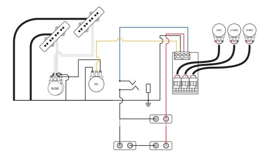
Blend, volume controls with bypass switch.
