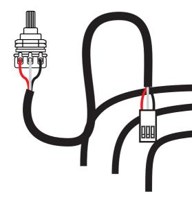
The cables should be mounted with the small triangle visible.
